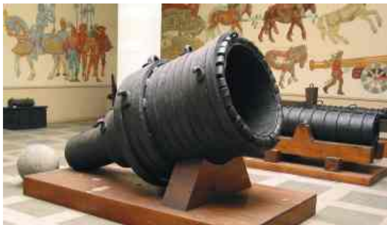
FIG. 4: PUMHART VON STEYR, FROM STYRIA, AUSTRIA, THE LARGEST-KNOWN (BY CALIBRE) WROUGHT-IRON MEDIEVAL BOMBARD. MORE THAN 2.5 METRES LONG, WITH A CONICAL BARREL OF DIAMETER 76–88 CM
